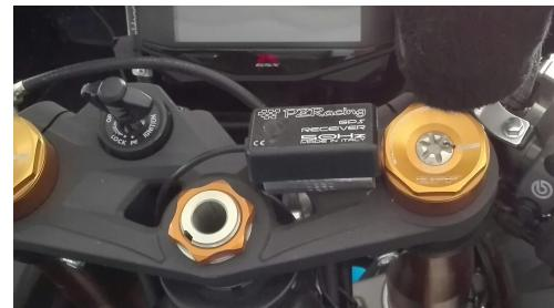
**Do not place the product on the tank fuel or the inner intakes of the bikes** because the GPS receiver would be fully covered by the body of the rider and his helmet or would be covered by the bike itself during a corner with high lean angle.
