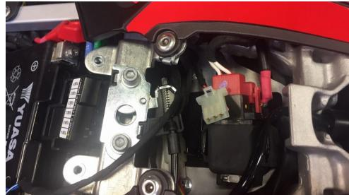
Place the receiver module with the writing facing upwards and in a horizontal position with a clear and unobstructed view of the sky, **it is recommended to place on the steering plate as horizontal as possible trying to avoid that is facing the pilot.**
